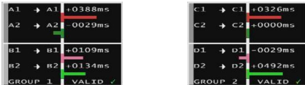
Figure 14 Eight Channel Delays
