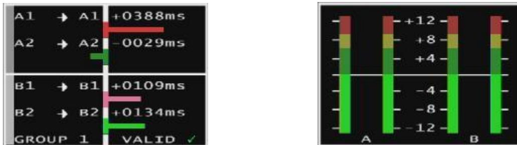
Figure 13 Four Channel Delay Meter and PPM Display
